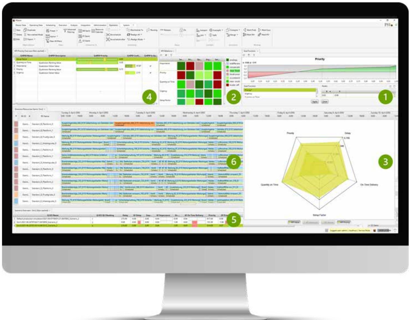
Figure 1: PSIasm/Qualicision with scenario selection, Qualicision scheduling, Goal Conflict Analysis and KPI optimization dashboard including goal achievement diagram and KPI setting functions as well as a Qualicision preference setting with the associated KPI achievement levels.
